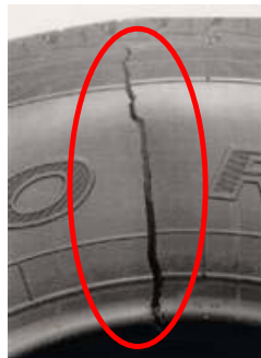
Bead wire is broken.
